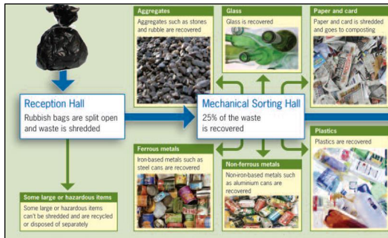
Figure 5: How an MBT plant works Source: Anon
